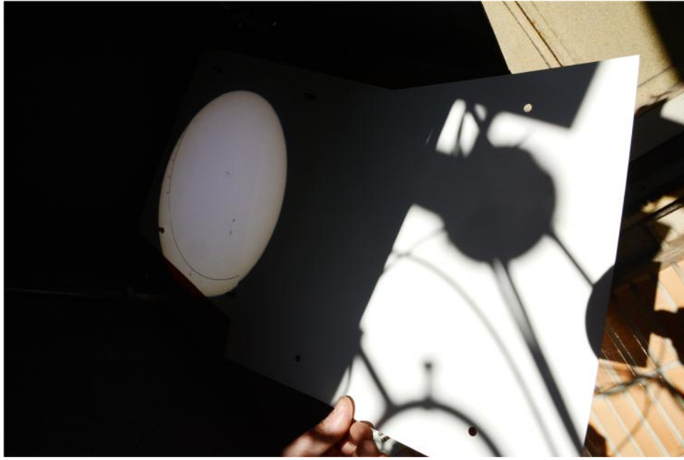
Figure B1. Sample picture showing the strong intensity contrast between the projected solar image and direct sunlight falling on an identical white projection sheet, as photographed at the Royal Observatory of Belgium (ROB) in Brussels on 2023 April 4 at 14:21 UT (picture courtesy of Olivier Boulvin). Here, the telescope has an aperture of 16 cm and it projects a 25 cm solar-disk image. This historical Merz–Grubb telescope from the late 19th century has been used for the sunspot drawings at the ROB since about 1885, and its optics are comparable to the instrument used by Carrington ( https://www.sidc.be/uset/telescopewvisual.php# ).
